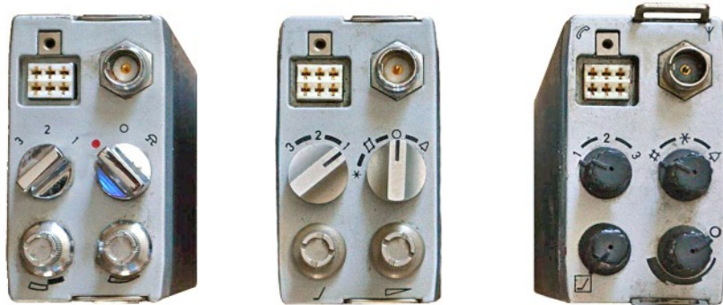
Three almost identical looking VHF FM radios: from left to right: VXW 020, PR 21 and PR 22. The knobs on the radios were different and identify a model at first glance: VXW 020 chrome plated, PR 21 aluminium and the PR 22 plastic. The functions differed slightly, for example the PR 22 volume control was in 3 fixed steps and the VXW 020 had not the Selectic option.
