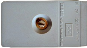
Bottom view of PR 21 or PR 22 (below) showing cover of battery compartment and covered socket for optional Selectic tone calling unit (above).
