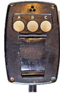
Standard speaker-microphone QK 065 05 (left), and type DX 28 (right) with three buttons for optional Selectic tone calling (right). Though fitted with the same type of plug, not each microphone of the VXW 100 and PR 22 series was interchangeable. Note the test lamp unit connected to the aerial socket.
